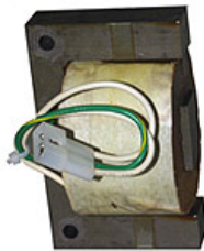
Electromagnets used in vibrator assemblies for sorting equipment.
