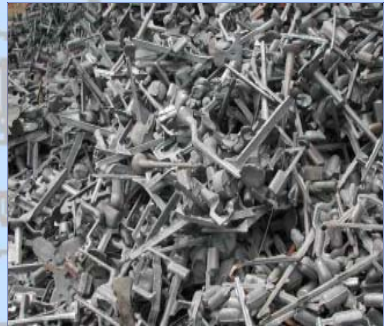
Shot blasted runners & risers to minimize slag generation
