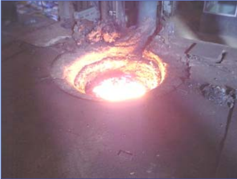
Furnace without hood
