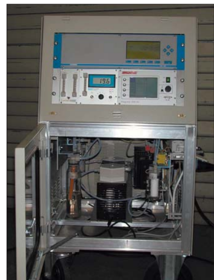
Figure 5. Mobile Flue Gas Analysing Measuring System.
